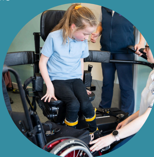
Swivel seat and swing away leg support, for manual transfer or transfer with hoist
