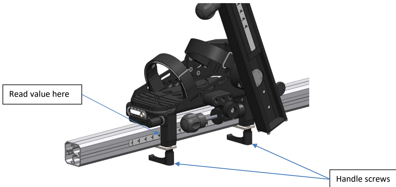
Picture 27. Position of the foot plate on the ski
